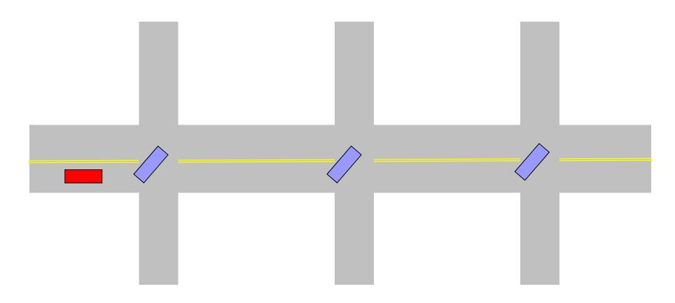
Used to mitigate delay to through traffic resulting from the cumulative impact of consecutive access points
